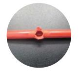
PAFSS fire suppression systems require no power for detection or operation. PAFSS fire detection tubing is installed throughout the risk area in the compartment, providing fast and effective detection of a fire. Upon flame impingement or high ambient temperature, the pressurised detection tube ruptures with a burst at the hottest point. The extinguishing agent is then discharged via the separate pipework and nozzles which are aimed at the identified risk within the compartment.
